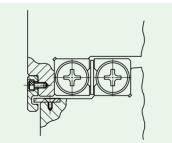
Fig. 5 Example of labyrinth seal
