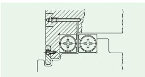
Fig. 4 Example of lubrication method
