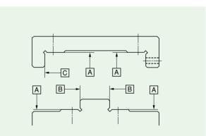
Fig. 7 Example of the mating mounting surfaces
