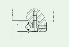
Fig. 3 Installation using the special mounting screw
