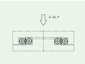
Fig. 2 Load rating direction
