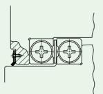
Fig. 6 Example of wiper seal
